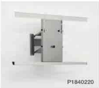
Electric lift for wall cupboards 400 to 1200mm wide. The diagonal adjustment has a single motor with two cross braces, allowing a cabinet to move down by 430mm and forward by 180mm.
