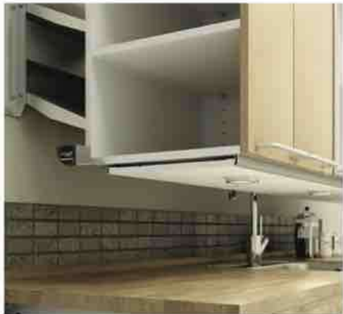
A pressure sensitive safety plate installed beneath the wall cabinets will suspend downward movement if resistance is encountered. The unit will then automatically rise by 10 to 30mm releasing tension between the safety stop and obstruction.
